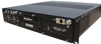
Figure 14 – TETRAPOL Radio Access Gate
