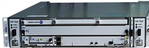
Figure 21 – Alcatel-Lucent 9773 LTE Micro Core detail
